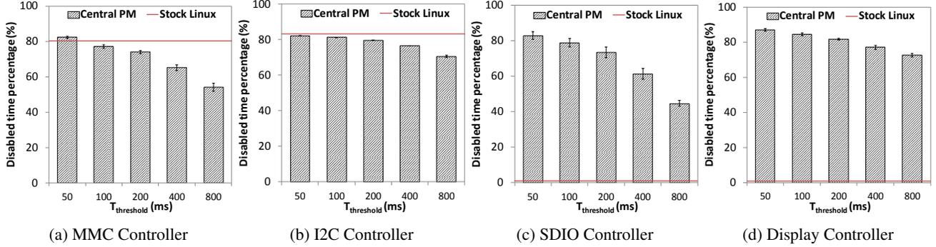
Figure 6: Device DISABLED time with different  $T_{threshold}$ , with the default being 100 ms in this paper. The Linux stock drivers in (a) and (b) come with hand-tuned PM code while that of (c) and (d) does not. In (c) and (d), we have slightly shifted up the lines for Linux stock drivers to make them visible since they are 0. With  $T_{threshold}=100$  ms, the central PM agent saves at most 17 mW by disabling (c) the SDIO controller, and 10 mW by disabling (d) the display controller.
