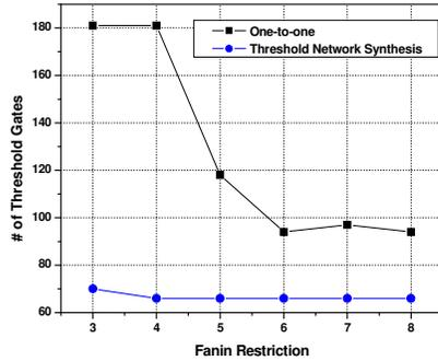
Fig. 10. Gate-count vs. fanin restriction for *comp*.
